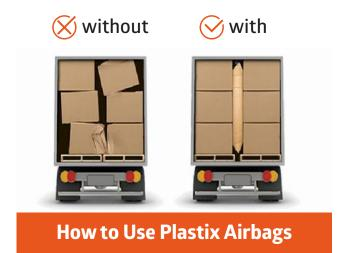
Position the airbag at least 1 inch above the floor,
